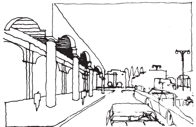
Fig. 8. To promote air circulation in street-side arcades design them with high canopies.
